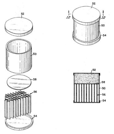
Figure 9 – Barrier Unit Physical Design – Option #2
