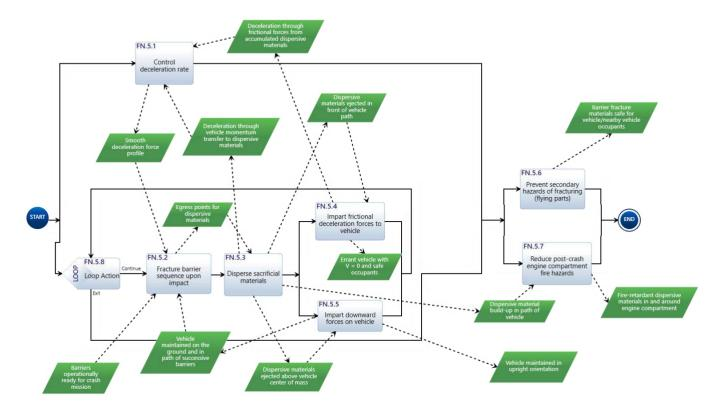
Figure 7 – Innoslate Action Diagram for Decelerate Errant Vehicle
