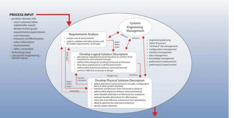
Note 1: The Systems Engineering Process is applied reportedly to nach design object, starting at, for example, the Capability, Mission or Use System, then to, for example, the Prime Mission or Use Product, Maintenance System, Production System, Operational Infrastructure, etc., them to subsystems of their systems.
