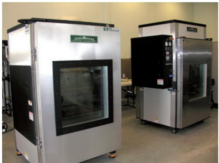
*Figure 3: Typical HALT chambers*
