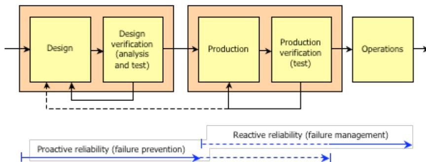
Figure 1: Verification of design and production
